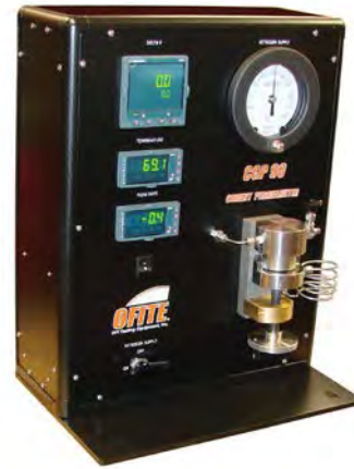
#120-87-DAS - Cement Permeameter with Data Acquisition System
