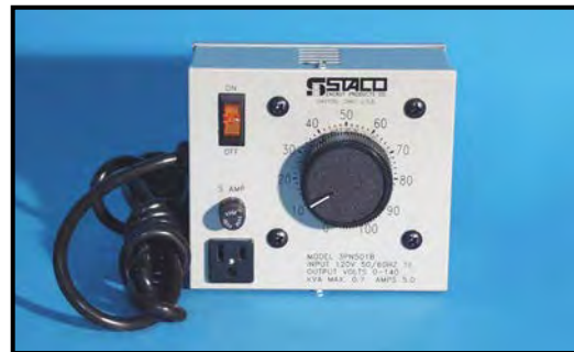
#152-35 - POWERSTAT® for 2-Speed Laboratory Mixer
