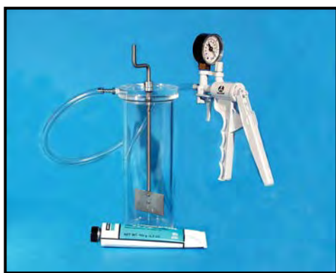
#110-00 - Mud Deaerator with Vacuum Pump
